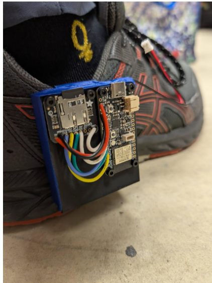
Figure 12: Original PLA hardware Case Inserted in Shoe
