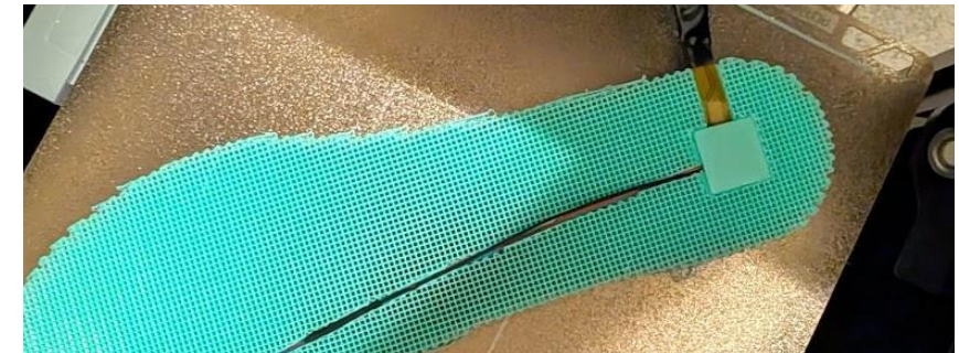
PCB inserted in 3D printed insole
