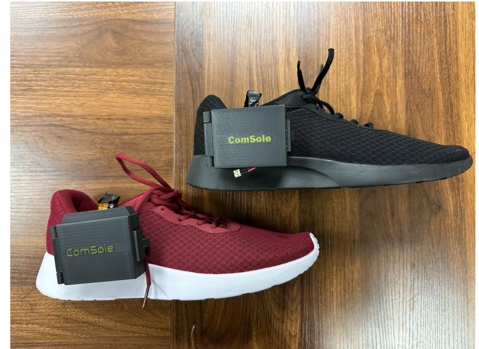
COMSOLE Product Installed In Test Shoes.
